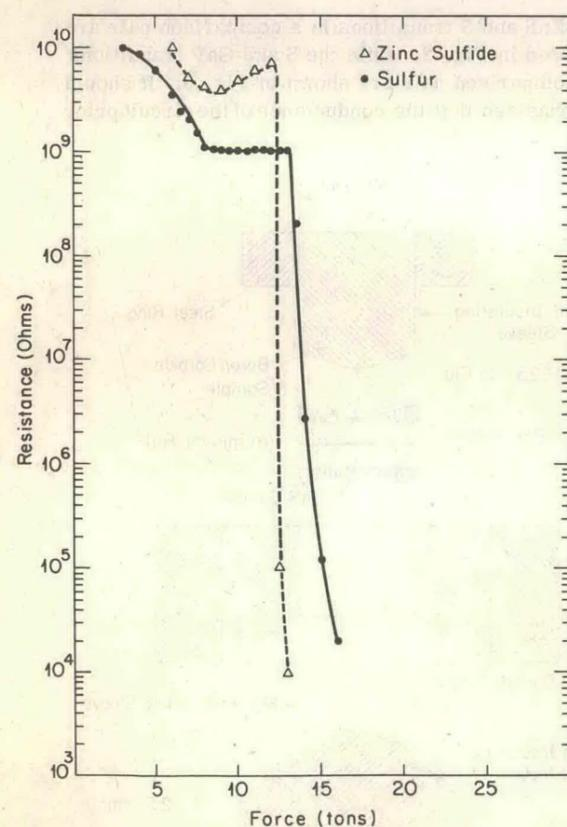
FIG. 2. Resistance versus force curves obtained simultaneously for ZnS and S. The resistance of the sulfur sample circuit prior to the transformation is primarily due to the gasket and other factors rather than due to the sulfur sample itself. After the transition the resistance value for the sulfur circuit is essentially entirely due to the sulfur.
